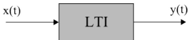
Figure 3.4: Linear Time Invariant (LTI) system with one input and one output.
